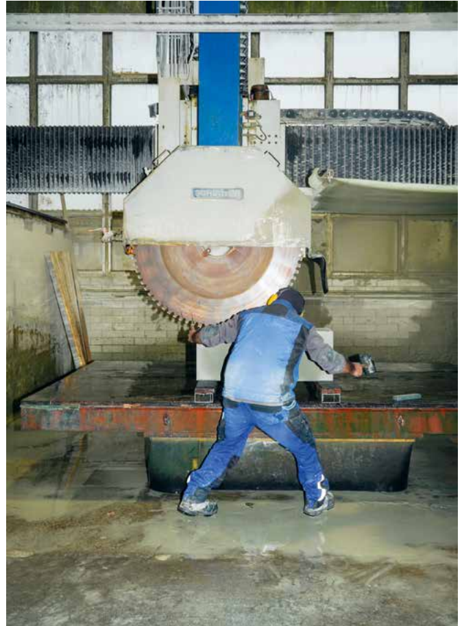
Blocks are cut up with the 'singing milling machine'.
